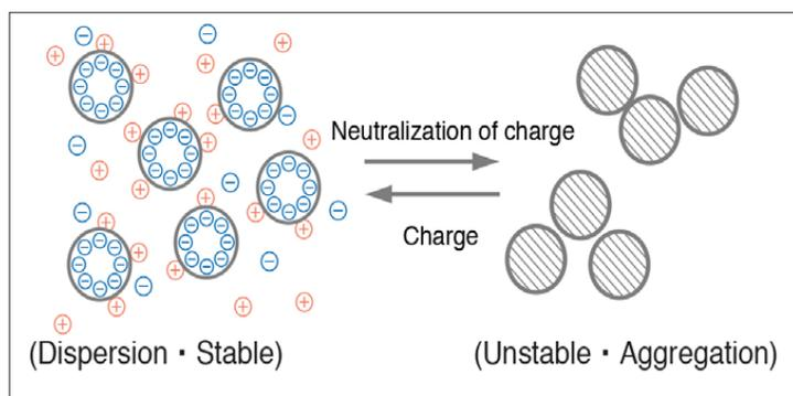
To measure zeta potential, a current is passed through the suspension and the electrophoretic mobility of the particles is measured by electrophoretic light scattering (ELS). Since it is difficult to pass a current through low polarity to non-polar organic solvent, i.e. low dielectric constants, an analysis cell must be optimized to make this measurement.
