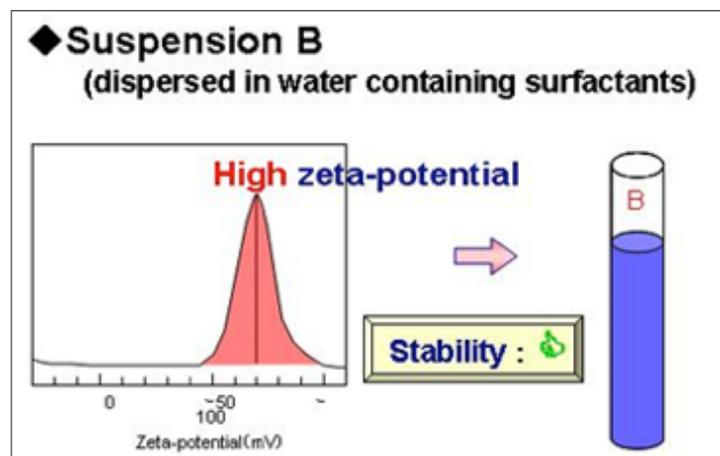
Zeta potential is measured by Electrophoretic Light Scattering (ELS). In ELS, the sample suspension is introduced into a specialized cell with two parallel electrodes. The electrodes generate an electric field and the particles will shift towards one electrode or the other. A laser with a known base frequency strikes the particles and a Doppler-shift in the frequency caused by the shifting particles is detected. A mobility is then calculated, from which a zeta potential can be calculated.
