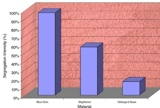
Figure 7. Segregation Intensity for laundry detergent with brightener
