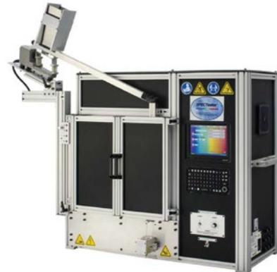
Figure 4. SPECTester used in Segregation Analysis
