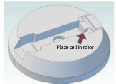
**Step 3:** The cell and rotor assembly are rotated to a prescribed speed and held for an allotted time. This causes centrifugal forces to act on the bulk material in the conical cell and compact the material within the cell. The rotor speed and the weight of the material, along with the position relative to the axis of rotation, are used to compute the consolidation pressure. Rotate to consolidate
