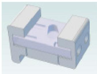
**Step 2:** A guard is inserted at the top of the cell and the cell is placed in the rotary cavity such that the axis of the conical cavity is 90 degrees from the direction of rotation.
